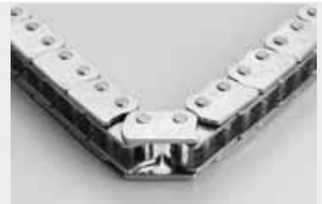
Telescopic chain end providing a rapid adjusting from 0 to 15mm, even with chain completely retracted into the actuator housing, that allows easy application on windows with overlap.
