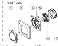
(5) Sensor housing 6 PCB module
