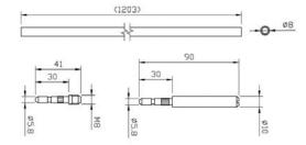
Zinc-plated rods for counterlock/flush bolt
