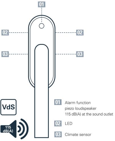
On account of its VdS-certified sensitivity, an ECO **ALERT** alarm window handle can also monitor multiple-casement windows. To guarantee a uniform appearance, we also supply window handles without alarm and climate function in the same high-grade design.
