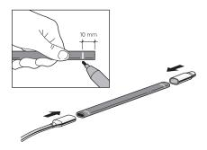
Measure off and mark a point exactly 10 mm from each end of the contact strip. Then slide on the end pieces up to the marks (tolerance ±1 mm).
