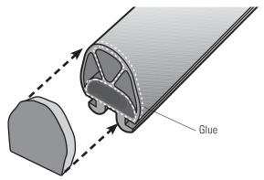
Attach end caps by applying ES-KLEBER to the points shown and hold in place, applying pressure across the whole area, for approx. 10 seconds. **Note:** No end caps on ELE040/081 and ELE040/105
