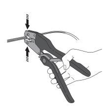
Using the crimping tool, crimp the end pieces at both ends and check they are secure. Squeeze pliers firmly together.
