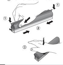
Moisten «click-fit foot» rubber profiles with a solution of soapy water and press into the aluminium profile (do not pull in).
