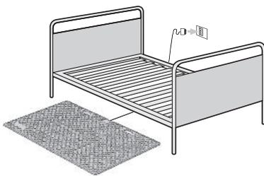
Position the CareMat® centrally in front of the bed so that avoiding the mat is impossible. Route the cable under the bed in order to avoid the risk of tripping over it. Insert the plug into the correct plug - socket device.
